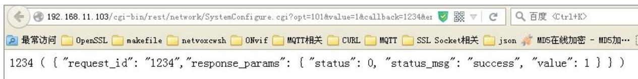
3. Users can switch Z202 Gateway mode back to Z207 mode through below cgi configuration.
