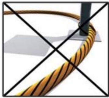
binding with metal (susceptible to interference)
