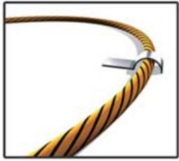
fixed by cable clips (recommend)
