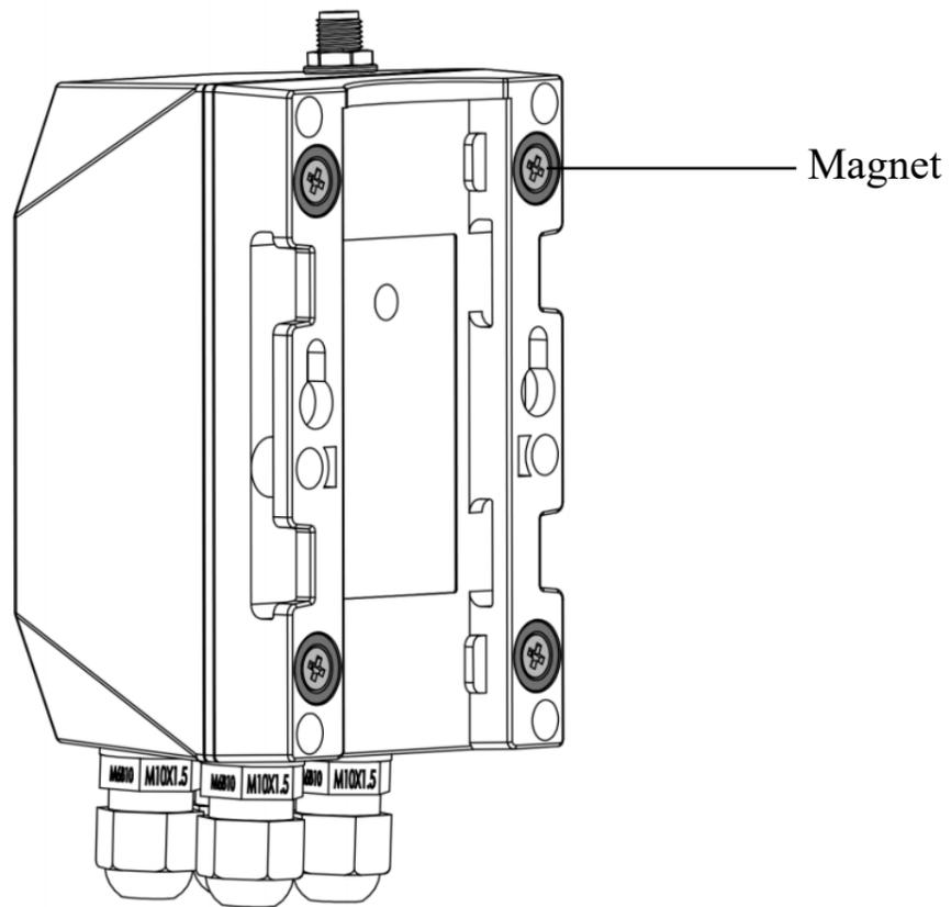
① Fix the R900 on a metal surface.
