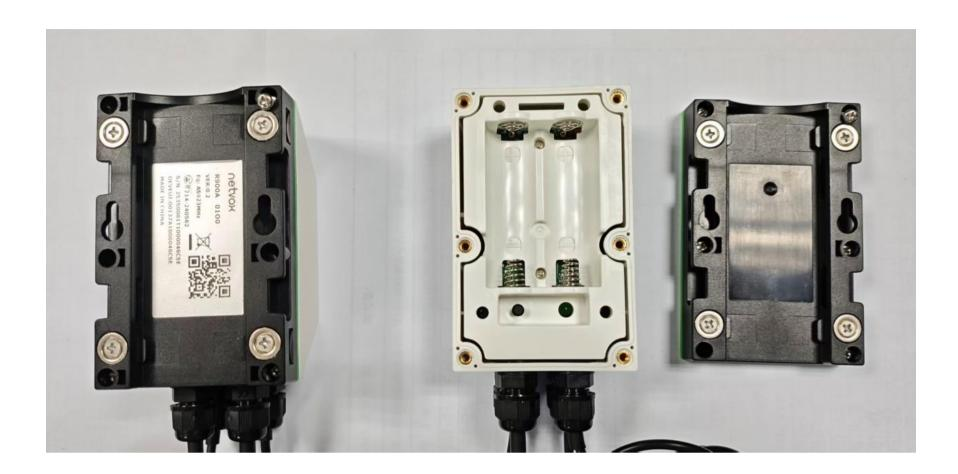
2 Install the battery, ensuring the correct polarity. After installation, reattach the rear cover and tighten the six screws securely.
