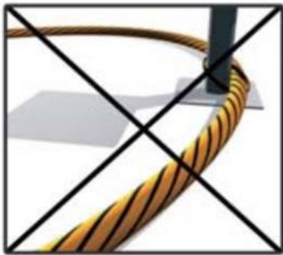
✗ Fixed with metal (may cause interference)
