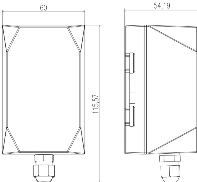
**Wireless Temperature Sensor - Digital Sensor with 1 x Digital Output****Electrical Specifications**
