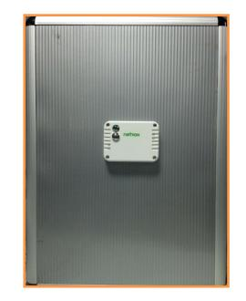
2. Temperature and humidity and article movement sensors detect temperature (or humidity) according to Min Time. When the detected temperature value (or humidity value) is compared with the last report, it exceeds the set value (temperature default 1 °C; humidity default 1%). , That is, the temperature change exceeds 1 ° C (or the humidity exceeds 1%), and the
