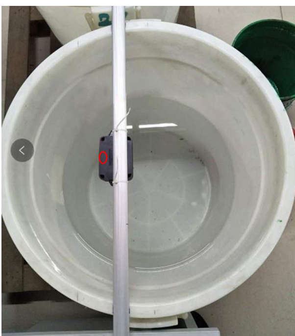
The probe offset center point 7cm
