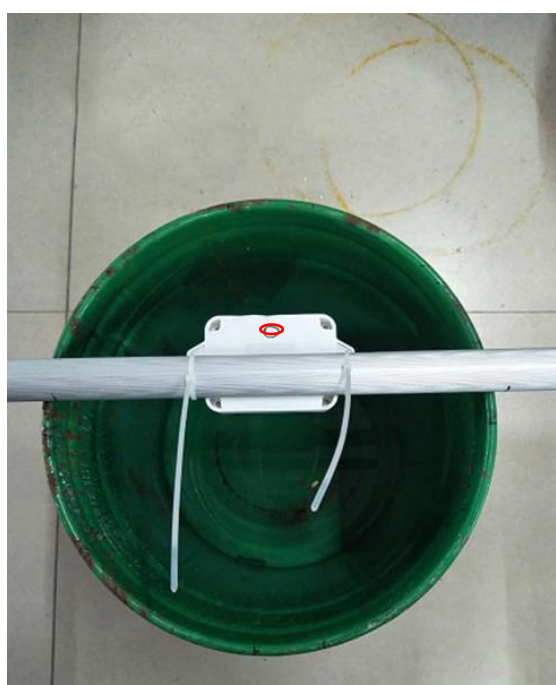
The probe offset center point 5 cm
