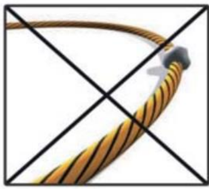
fixed by glue (susceptible to damage cable)
