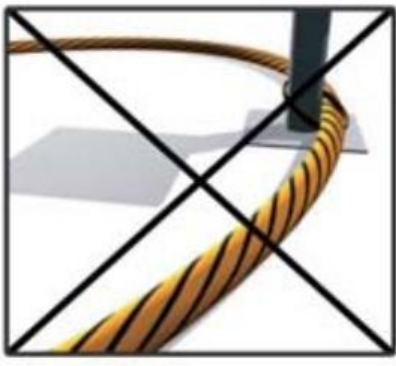
binding with metal (susceptible to interference)
