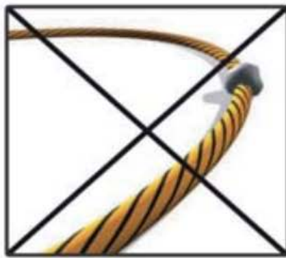
fixed by glue (susceptible to damage cable)
