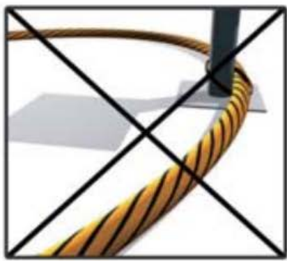
binding with metal (susceptible to interference)
