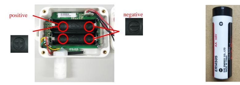
Step 3: After inserting the batteries, put the lid back on and tighten the four screws.
