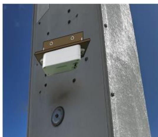
Figure 1. Install the device upside down.
