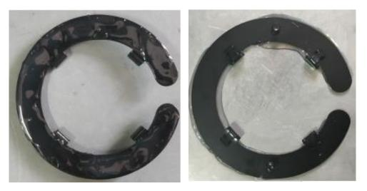
Step 10. Clean the dirt or coupling gel on the surface of the probe.
