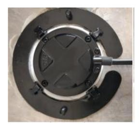
Step 13. Install and cross spring hooks on the lid.
