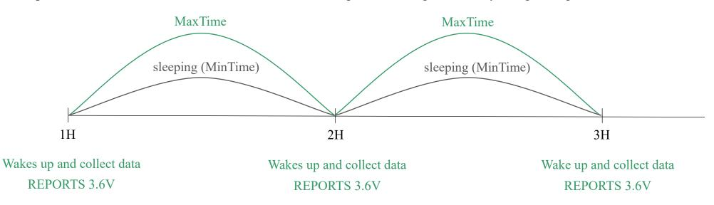
Example#1 based on MinTime = 1 Hour, MaxTime= 1 Hour, Reportable Change i.e. BatteryVoltageChange=0.1V
