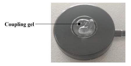
Step 5. Tap the sensor on the surface of the container and test if it reports data.
