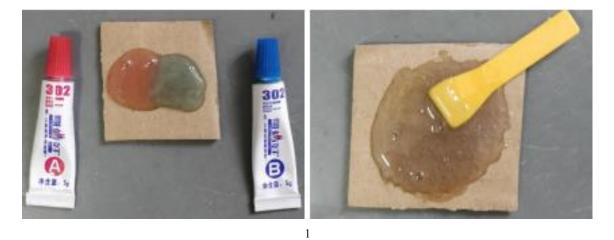
Step 8. Apply the AB glue to the bottom of the holder.
