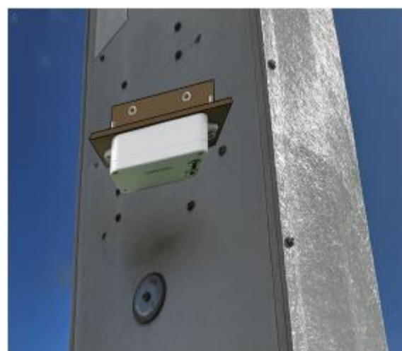
Fig 2. Install with LED and function key faced downwards
