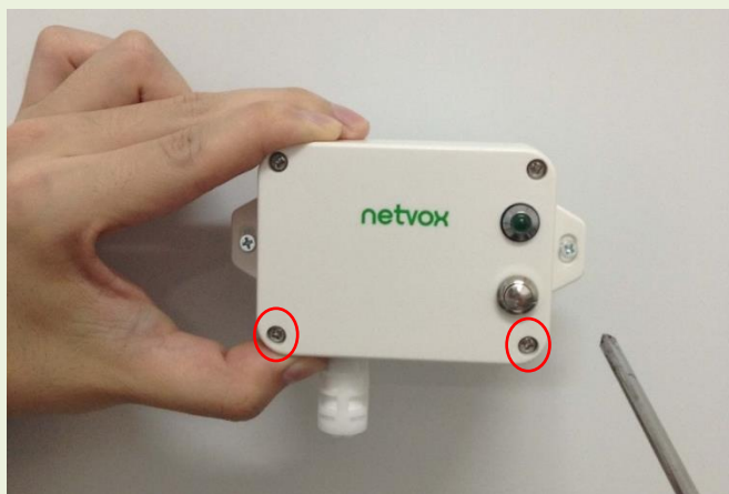
Screw hole diameter: Ø4mm
