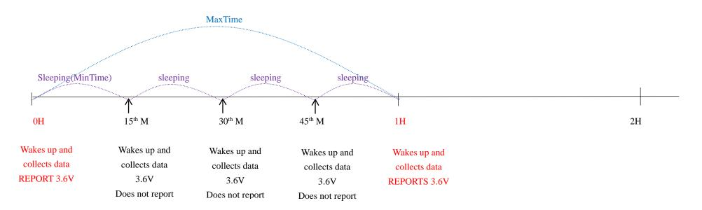
**Example#3** based on MinTime = 15 Minutes, MaxTime= 1 Hour, Reportable Change i.e. BatteryVoltageChange= 0.1V.
