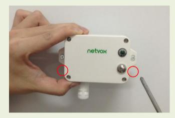
Screw hole diameter: Ø4mm
