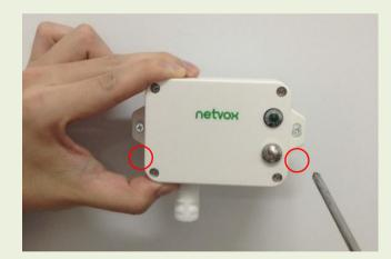
Screw hole diameter: Ø4mm
