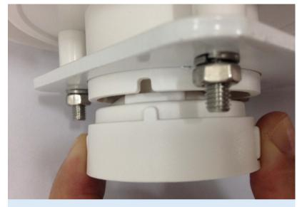
Press the buttons on both sides of the base, then gently take out the sensor inside the housing.
