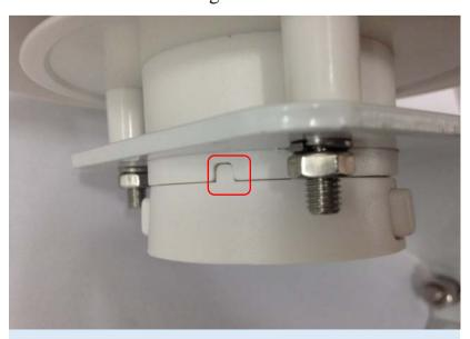
Note that the protruding part of the base should be aligned with the concave part of the housing.
