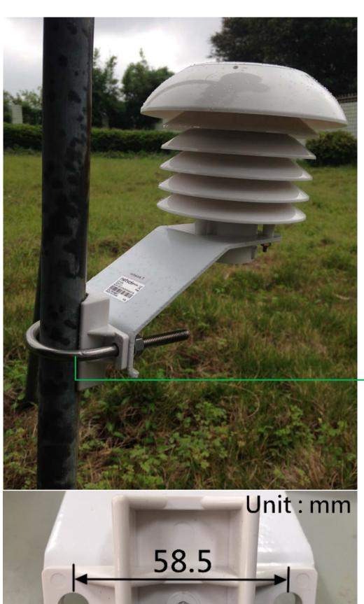
Range of diameter of post for mounting  $\emptyset 25 \sim \emptyset 50 \text{(mm)}$
