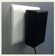
4. The device is compatible with the LoRaWAN open protocol Class C class device, which supports four kinds of sound and mute functions such as fire alarm, emergency, burglar, doorbell and the like through the downlink command control device; and also supports the LED light function: flowing light, blink and unlighted
