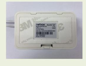
2. Remove the backing from the bottom of the sensor probe and attach it to a flat ground where water leakage may occur.
