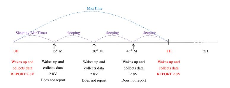
Example#3 based on MinTime = 15 Minutes, MaxTime= 1 Hour, Reportable Change i.e. BatteryVoltageChange= 0.1V.
