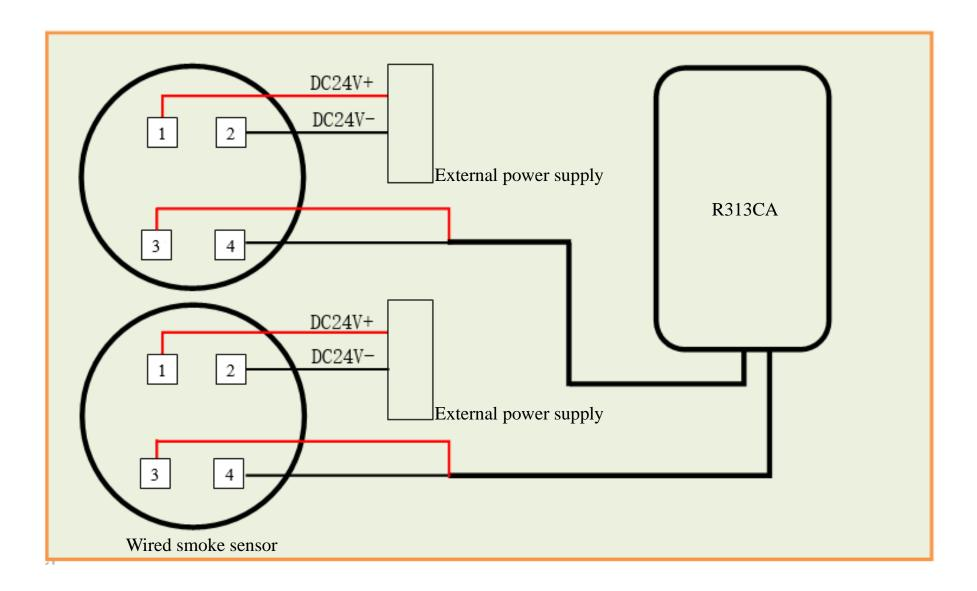
Fig. Diagram of connecting with the wired smoke sensor
