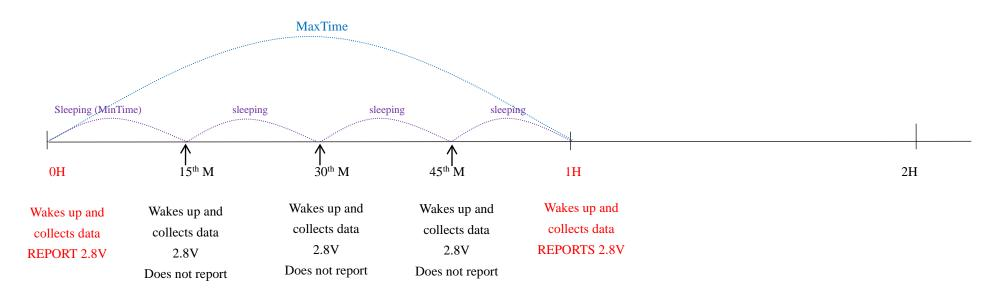
**Example#2** based on MinTime = 15 Minutes, MaxTime= 1 Hour, Reportable Change i.e. BatteryVoltageChange= 0.1V.
