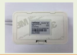
The figure shows that the water immersion sensor (R311W) is used in bathing rooms where there is a possibility of water leakage in the pipeline.
