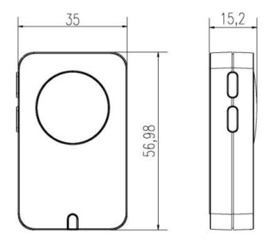
Figure 2 Dimensions of main engine shell
