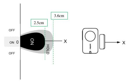
If the magnet moves along the Y axis relative to the sensor, it will cause repeated reports due to the magnetic field.
