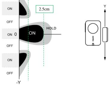
1.Tear off 3M release paper of the magnet body and attach the body to the door frame and stick it to the door in parallel with the door magnet body. (please do not stick it on the rough door to avoid falling off after using the device for a long time).
