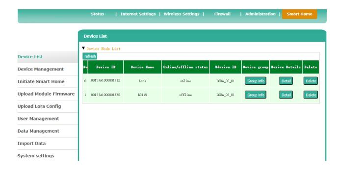
5. After the deletion is successful, click the restart button in the upper right corner to restart the gateway once and the replacement can be successful.
