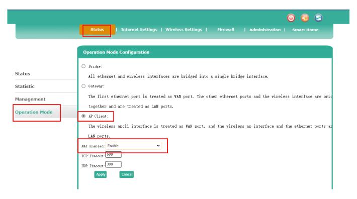
5. After the webpage is reconnected, click [Wireless Settings] → [AP Client] to view the WiFi channel of the router to be bridged in the WiFi list.
