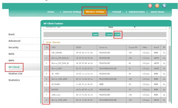
6. Enter the WiFi information of the router to be bridged (including WiFi name, Mac address, security mode, encryption method, WiFi password, etc.) in the [AP Client Feature] item, and then click [Apply]
